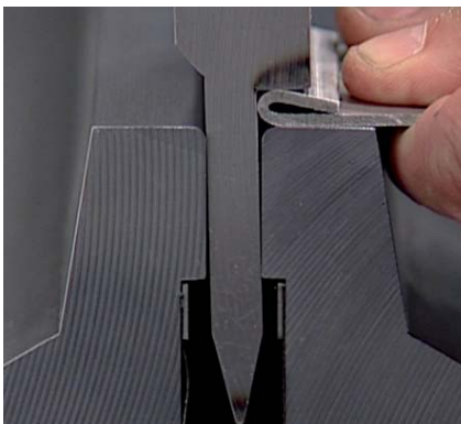
Pre-bend and flattening in the same tool.
