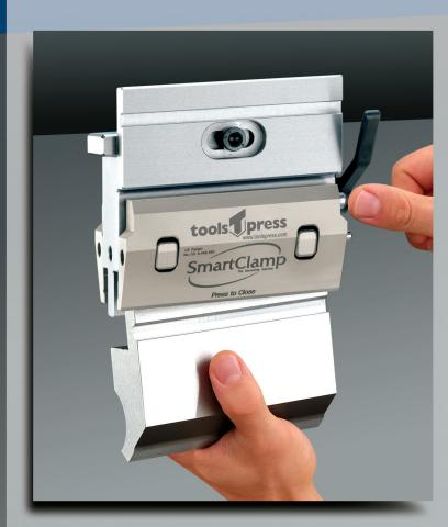
To load the punch, insert it to the top, press in a simple way the locking clamp plat to the front and use the locking lever to reference and seat the punch directly. Using Smart Clamp, you can safely and confidently load and remove any punch section from the front of the machine.
